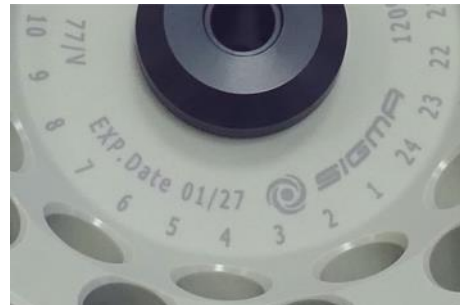
Fig. 7: Different service life – engraving on the bucket/rotor
