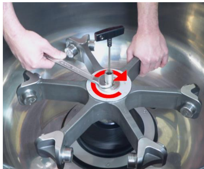
Fig. 13: Fastening of the rotor
