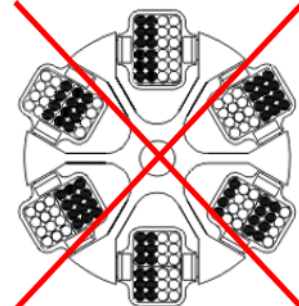
Fig. 15: Permissible and impermissible loading of an angle rotor and a swing-out rotor (example illustration)
