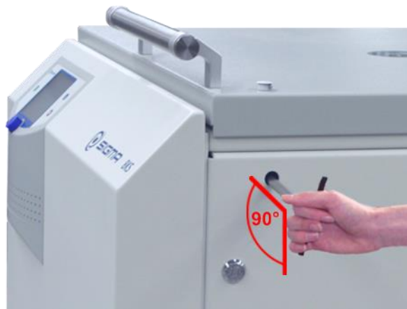
Fig. 40: The emergency lid release key must be inserted horizontally.
