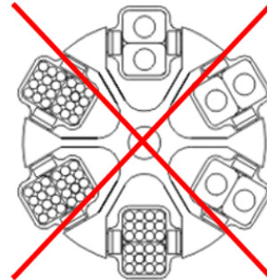
Fig. 14: Permissible and impermissible loading of a swing-out rotor with vessels of various sizes (example illustration)
