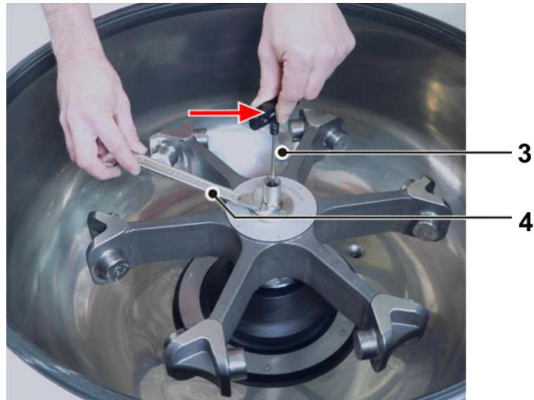
Fig. 12: "Two-finger-principle" for holding the hexagon key
