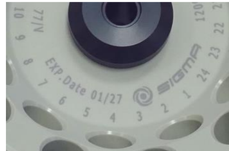
Fig. 7: Different service life – engraving on the bucket/rotor
