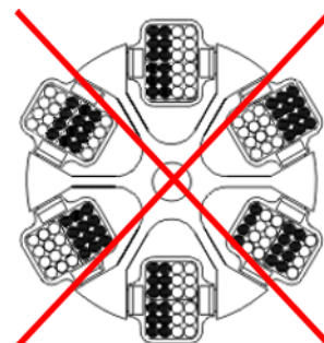
Fig. 15: Permissible and impermissible loading of an angle rotor and a swing-out rotor (example illustration)
