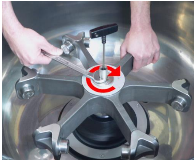
Fig. 13: Fastening of the rotor
