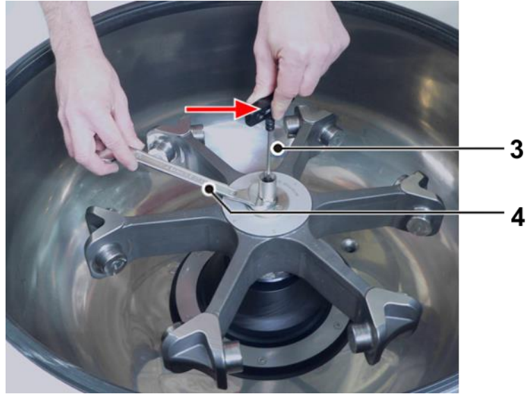
Fig. 12: "Two-finger-principle" for holding the hexagon key
