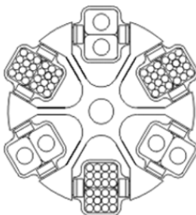
Fig. 10: Permissible and impermissible loading of a swing-out rotor with vessels of various sizes (example illustration)
