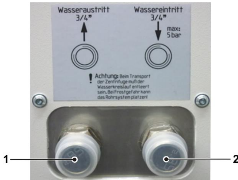
Fig. 8: Connections for the cooling water system
