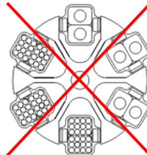
Fig. 10: Permissible and impermissible loading of a swing-out rotor with vessels of various sizes (example illustration)
