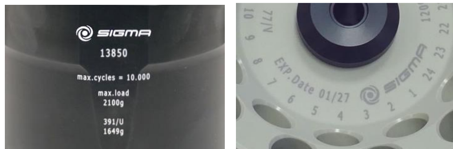
Fig. 4: Different service life – engraving on the bucket/rotor
