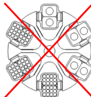
Fig. 8: Permissible and impermissible loading of a swing-out rotor with vessels of various sizes (example illustration)
