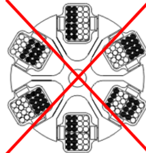
Fig. 9: Permissible and impermissible loading of an angle rotor and a swing-out rotor (example illustrations)
