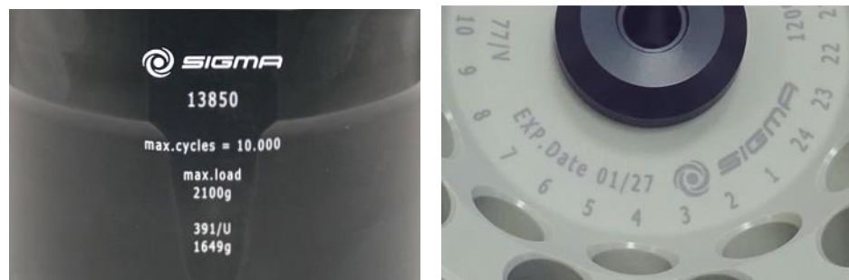
Fig. 4: Different service life – engraving on the bucket/rotor
