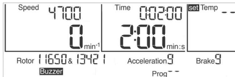
Fig. 19: Display with a deactivated temperature monitoring function
