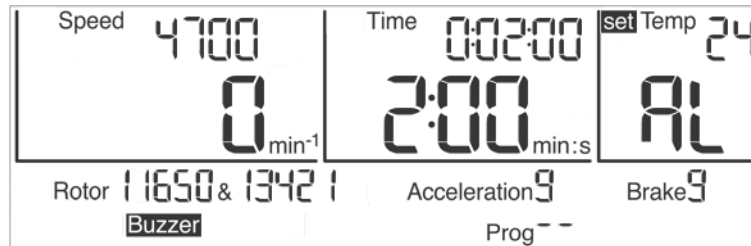
Fig. 20: Display with an activated temperature monitoring function
