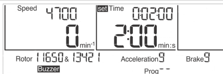
Fig. 15: Setting the runtime, here in the time unit "min:s"
