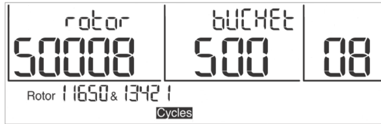
Fig. 28: Display when the maximum number of cycles is reached (flashing)
