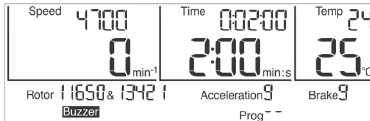
Fig. 21: Indication (maximum value, flashing) when the alarm temperature is exceeded
