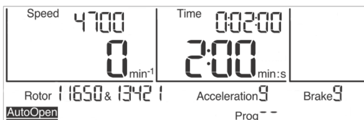
Fig. 24: The automatic lid opening function "Auto Open" is activated
