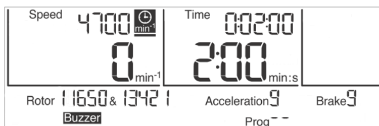
Fig. 16: The function "Runtime as of the set speed" is activated
