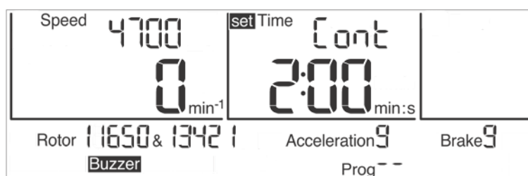
Fig. 17: Indication "Cont" during a continuous run
