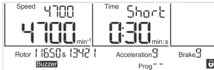
Fig. 18: Indication "Short" during a short run
