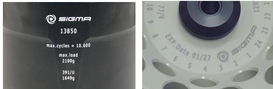
Fig. 4: Different service life – engraving on the bucket/rotor
