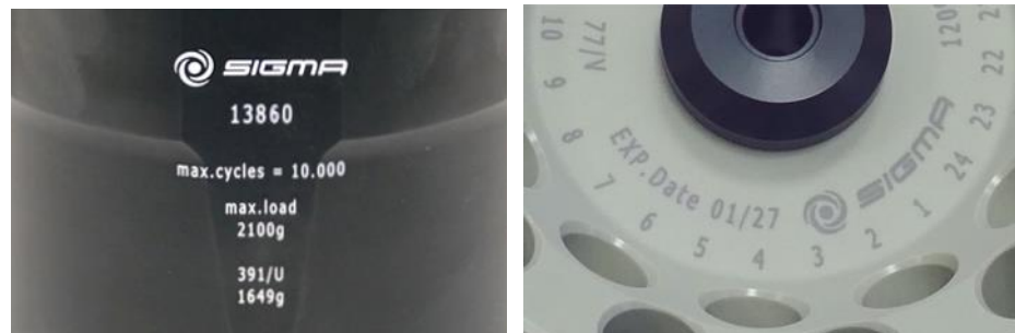
Fig. 5: Different service life – engraving on the bucket/rotor
