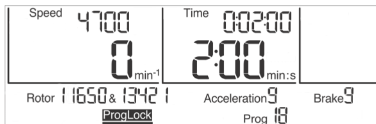
Fig. 26: The program lock "ProgLock" is activated
