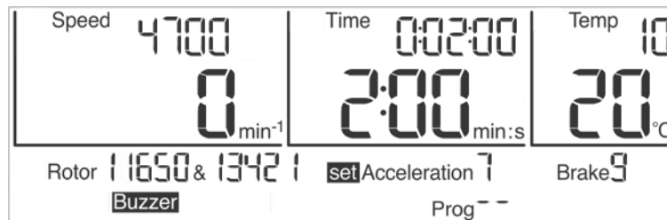
Fig. 21: Preselection of a curve; here: preselection of an acceleration curve
