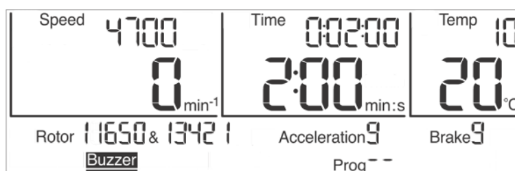
Fig. 24: The sound signal "Buzzer" is activated
