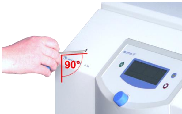
Fig. 35: The emergency lid release key must be inserted horizontally (example illustration)
