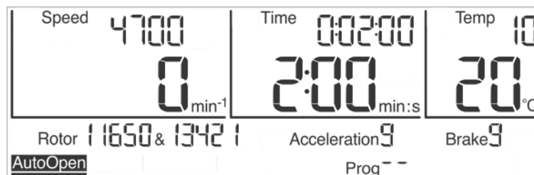
Fig. 23: The automatic lid opening function "Auto Open" is activated
