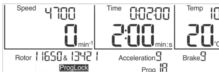
Fig. 25: The program lock "ProgLock" is activated
