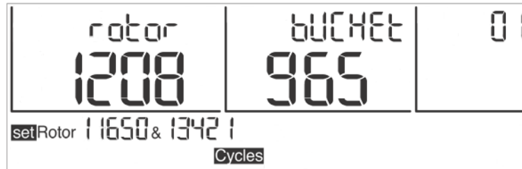
Fig. 26: Cycle display for rotor 11650 and bucket 13421
