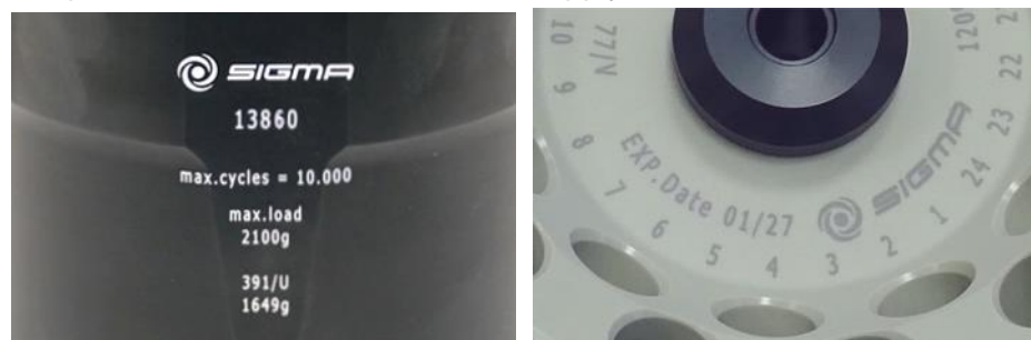
Fig. 6: Different service life – engraving on the bucket/rotor
