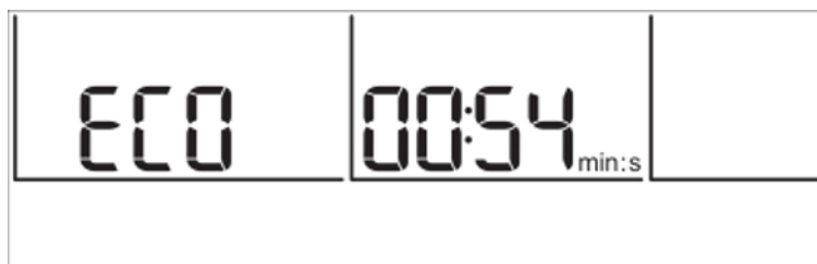
Fig. 29: Indication of the last 29 minutes of the countdown before the activation of the Eco mode
