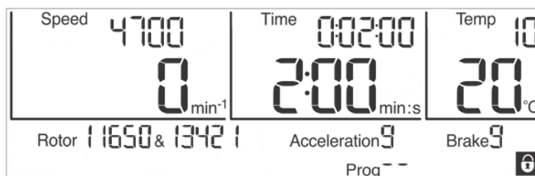
Fig. 28: "Padlock" symbol indicating an activated input lock
