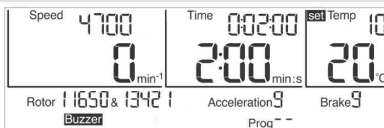
fig. 19: Setting the temperature
