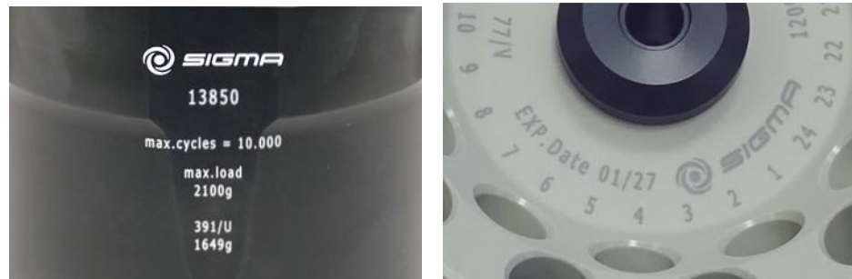
Fig. 5: Different service life – engraving on the bucket/rotor
