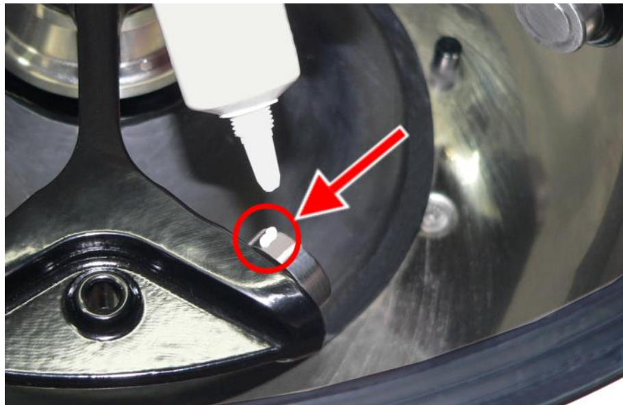
Fig. 32: Sufficient quantity of grease for one bolt
