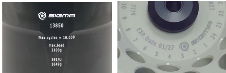
Fig. 4: Different service life – engraving on the bucket/rotor
