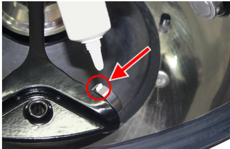
Fig. 33: Sufficient quantity of grease for one bolt
