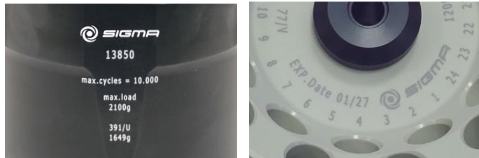
Fig. 4: Different service life – engraving on the bucket/rotor
