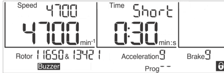
Fig. 17: Indication "Short" during a short run
