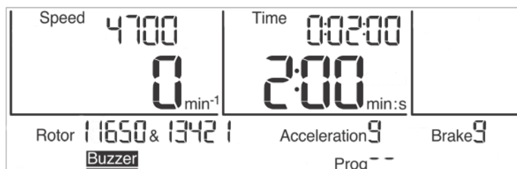
Fig. 21: The sound signal "Buzzer" is activated
