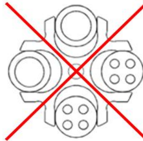
Fig. 8: Permissible and impermissible loading of a swing-out rotor with vessels of various sizes (example illustration)
