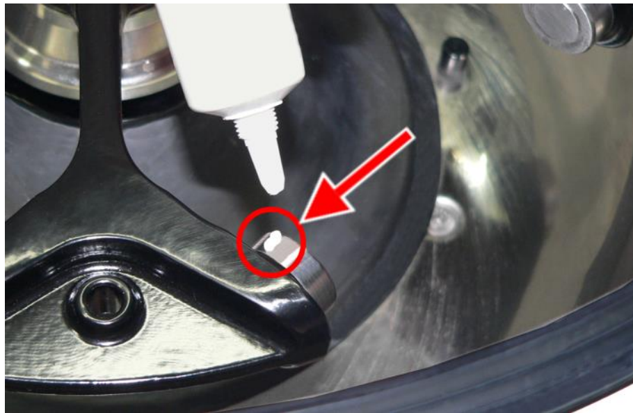
Fig. 31: Sufficient quantity of grease for one bolt
