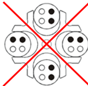
Fig. 9: Permissible and impermissible loading of an angle rotor and a swing-out rotor (example illustrations)
