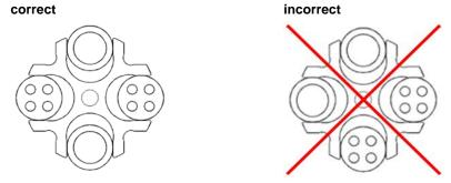
Fig. 6: Permissible and impermissible loading of a swing-out rotor with different tube sizes (example illustration)
