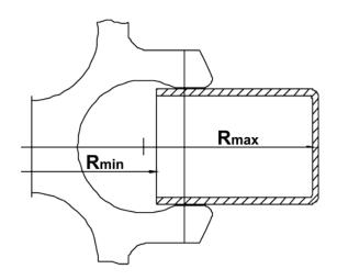
Fig. 14: Minimum and maximum radius of a swing-out rotor
