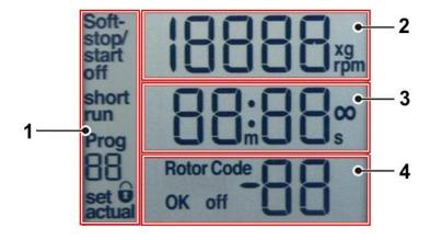
Fig. 10: Display, completely illuminated
