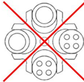
Fig. 6: Permissible and impermissible loading of a swing-out rotor with vessels of various sizes (example illustration)
