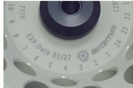
Fig. 4: Different service life – engraving on the bucket/rotor
