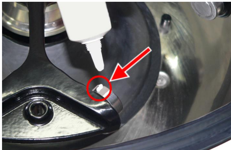
Fig. 29: Sufficient quantity of grease for one bolt
