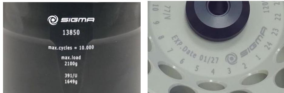
Fig. 4: Different service life – engraving on the bucket/rotor
