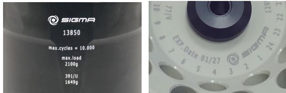
Fig. 4: Different service life – engraving on the bucket/rotor
