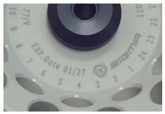
Fig. 4: Different service life - engraving on the bucket/rotor
