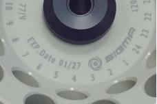
Fig. 5: Different service life - engraving on the bucket/rotor
