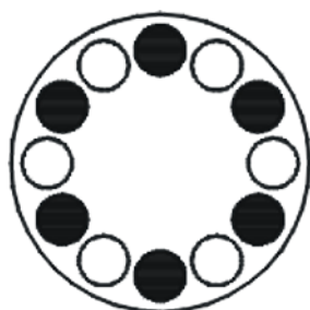
Fig. 11: Permissible and impermissible loading of an angle rotor (example illustration)
