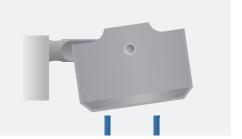
Three metal pins emerge from the chamber bottom and raise the bucket slightly to achieve exact positioning.
