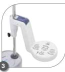
Robust electrode holder provides secure, smooth electrode movement throughout the measurement process.
