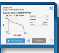
Automated titrant delivery system with high-accuracy burette and dispenser provides consistent results and automatic results calculations simplifies analysis and reduces computational errors.
