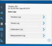
Internal data storage maintains a history of sample titrations, titrant standardizations, electrode calibrations and direct measurements – all with date and time stamp – to preserve critical data and facilitate easy data transfer to an external device.
